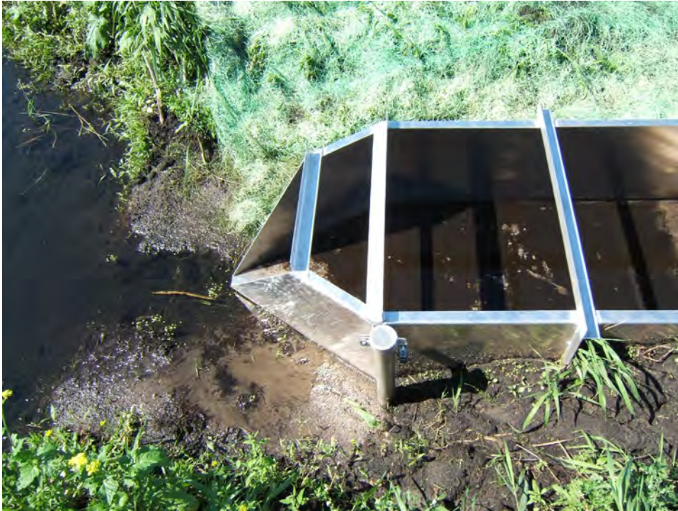
Figure 5. H-Flume for Surface Flow Measurement at the Bachand Site
