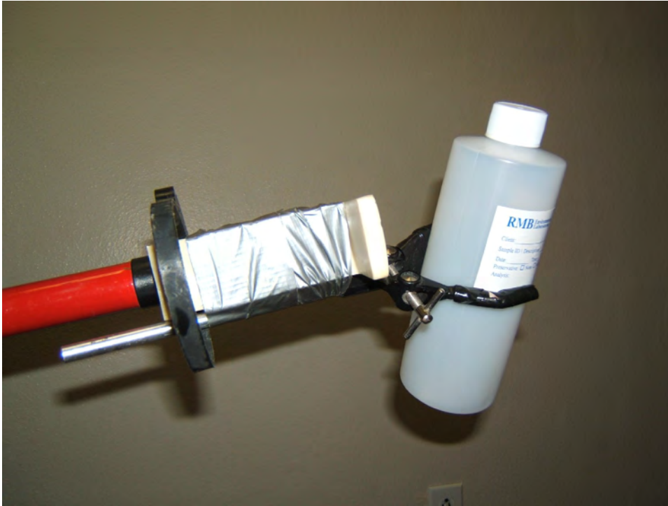
Figure 25. Clamp Attached to Sludge Nabber for Extended Dip Sample
