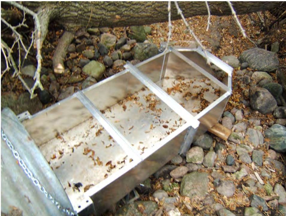
Figure 8. H-Flume on Downstream End of Yaggie 2 Culvert
