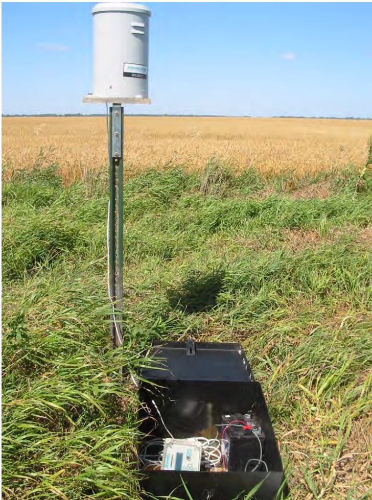
Figure 27. Rainfall Monitoring Station at the Bachand Site
