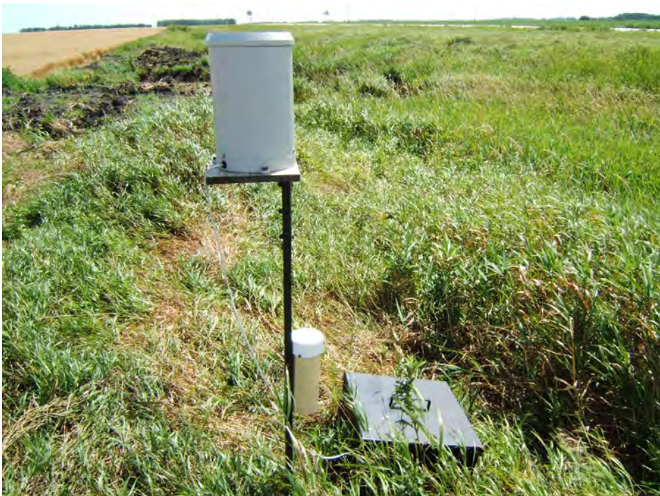
Figure 6. Rainfall and Barometric Pressure Monitoring Equipment at the Bachand Site
